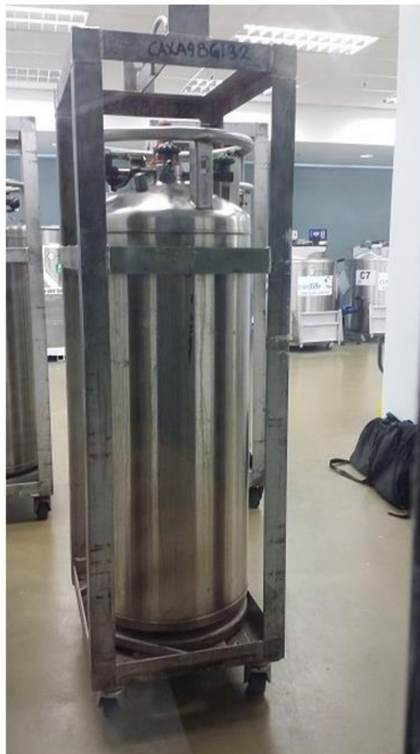
Individual pouches of blood samples are stored under cryogenic temperatures (under -150deg) in these vacuum insulated cryogenic storage tanks.
